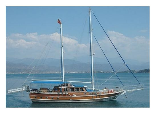
Type: Ketch Loa: 20.00 m. Beam: 5.70 m Engine: 450 hp Iveco
